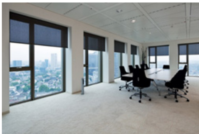
Figure 41: Internal shading system
