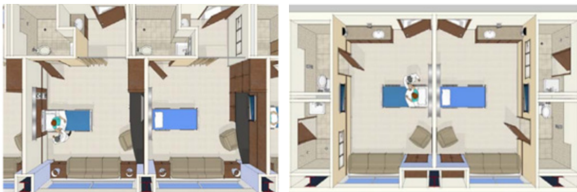
Figure 11: Patient room layout examples: Inboard same handed (top) and outboard opposite handed (right)
