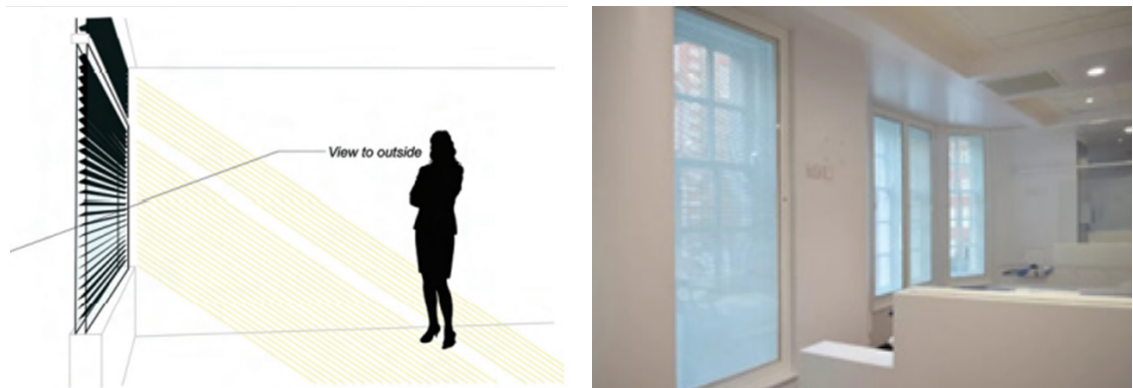
Figure 40: Operable louvres located between glass
